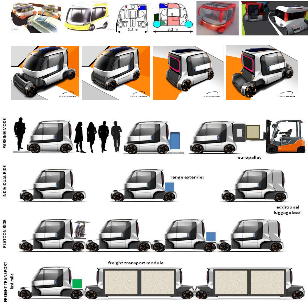
FIGURE 5 SEVERAL DESIGN PICTURES OF A COUPEMOBILE AND ITS POSSIBILITIES
