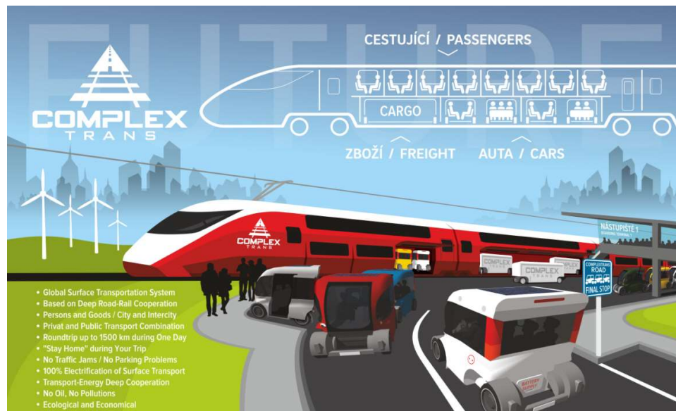
FIGURE 1 PLATFORM OF THE COMPLEXTRANS SYSTEM: PASSENGERS CHANGE (UPPER DECK) AND LOADING AND UNLOADING OF ADAPTED CARS (COUPEMOBILES) WITH PASSENGERS AND FREIGHT MODULES (LOWER DECK) IN THE COMPLEXTRANS TRAINS
