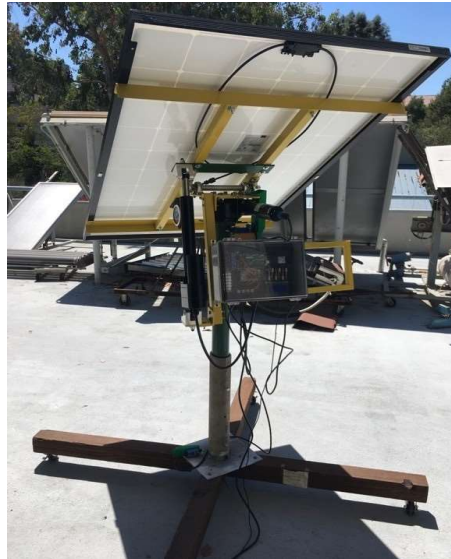
FIGURE 1 DUAL-AXIS SOLAR TRACKER WITH AUTOMATED CONTROLS BUILT BY A SUMMER UNDERGRADUATE RESEARCH TEAM IN 2018
