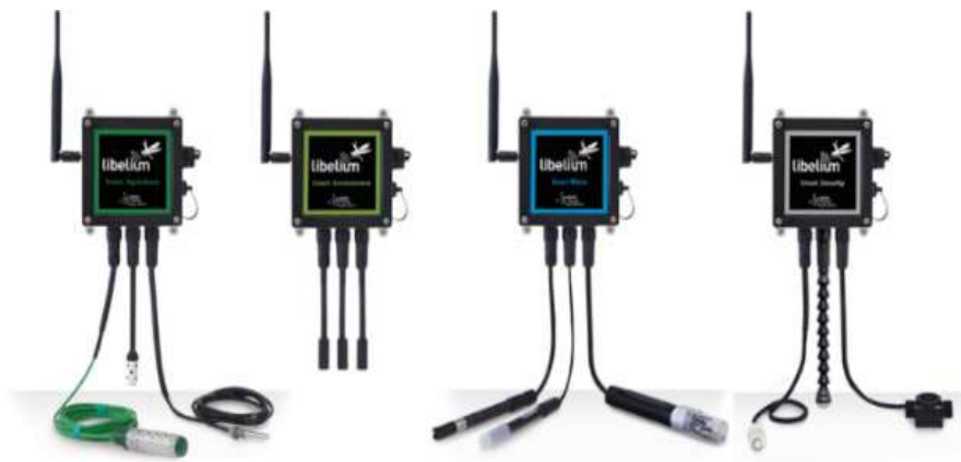
FIGURE 2 LIBELIUM SMART AGRICULTURE, WATER, ENVIRONMENT, AND SECURITY MODELS USED IN THE UQ SMART CAMPUS INITIATIVE 2016
